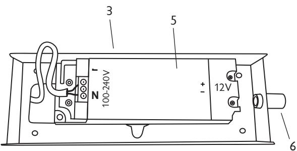
4. Kabelklemme anschrauben/ Screw on cable clamp/ Visser le
